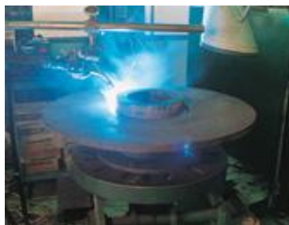
Automatic CO 2 / MIG welding process for Hub and End Disk.
