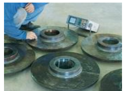
UT inspection for full-penetrated weld.
