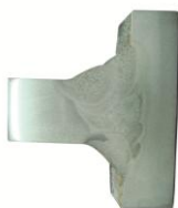
Weld between Disk and Shell
